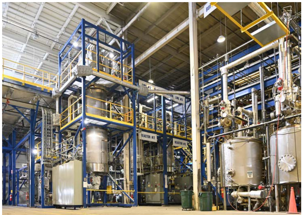
GreenMantra recycling technology converts plastics with short life cycles in their original applications to specialty polymers that act as process aids in products with long service lives. Courtesy of GreenMantra Technologies
