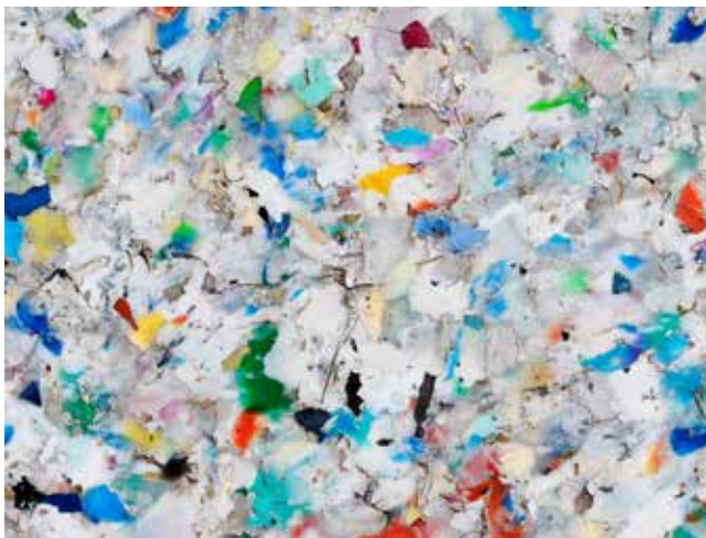
Fig: 1: Natural post-consumer HDPE bottle flake
