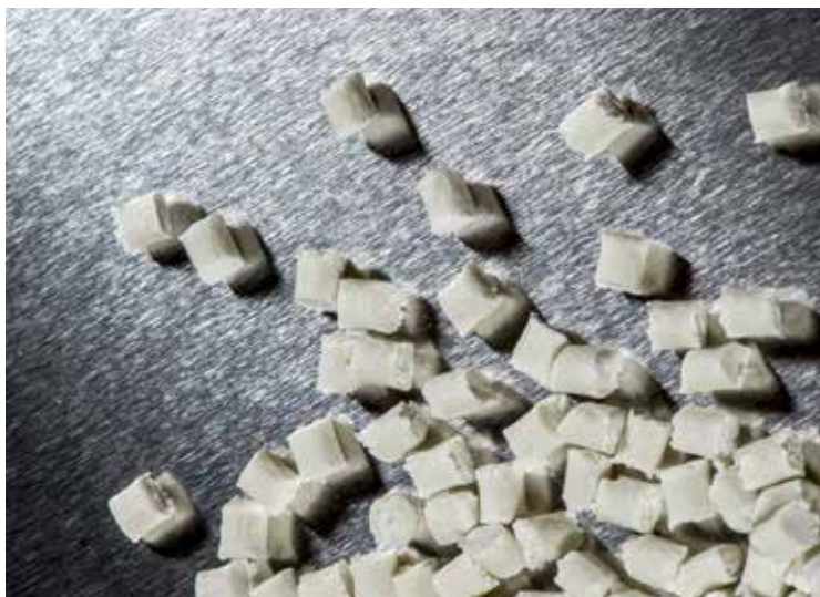
Fig 2: Natural HDPE flake reprocessed to pellet using Ceranovus A120 additive
